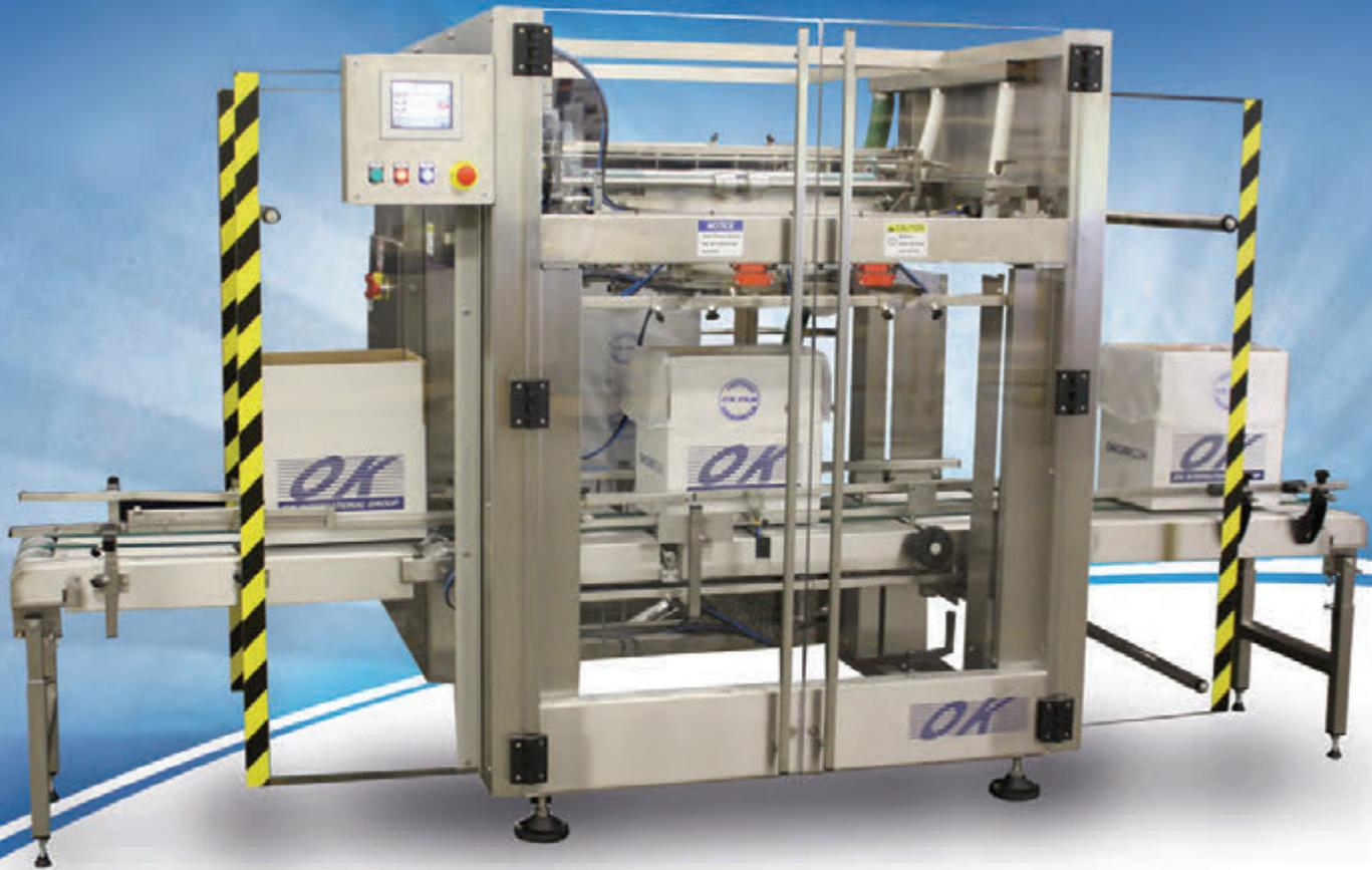
The Superliner SL220 case liner makes bags from a roll of gusseted polyethylene tubing, places the bag into a case, crate, drum or tray and cuffs the bag over the edges. The Superliner SL220 Servo case liner sets a new industry standard with a speed of up to 24 cases per minute.
