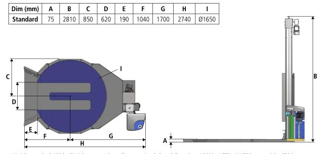
Weight, standard: 480 kg (Weight can vary depending on options). Crated dimensions: L2900 x H750 x W1700 mm, weight: 650 kg.
