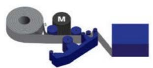
Pre-stretch system by fixed gear ratios. Adjustable to 150%, 200% and 250%.
